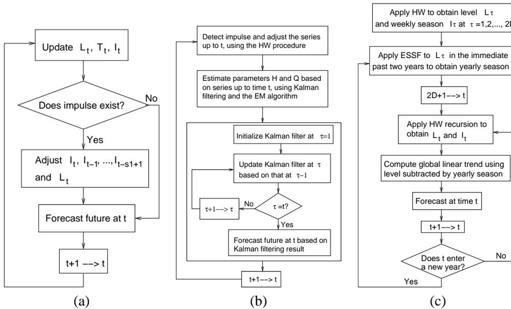
Figure 2: The schematic diagrams for the forecasting algorithms: (a) Holt-Winters with impulse detection; (b) GLS; (c) ESSF.
