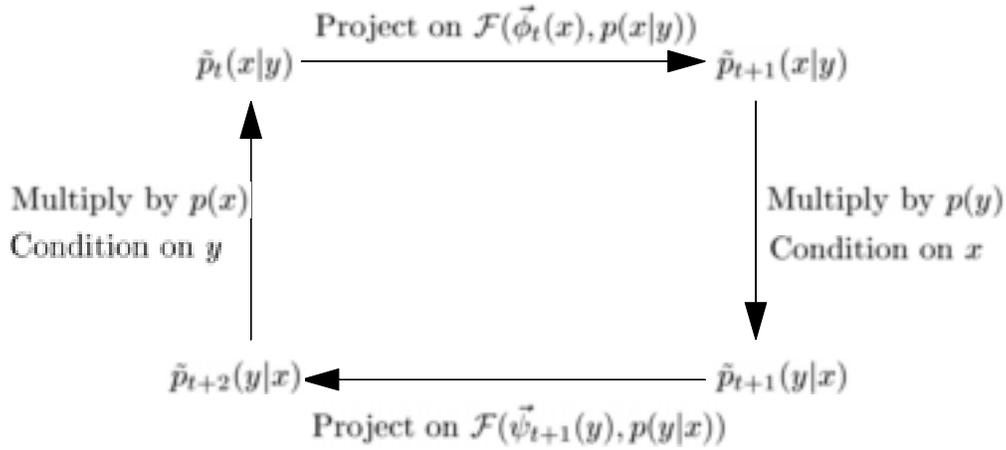
Figure 2: The iterative projection algorithm: The dual roles of the projections that determine  $\vec{\psi}(y)$  and  $\vec{\phi}(x)$  as dual Lagrange multipliers in each iteration. These iterations always converge and the diagram becomes commutative.
