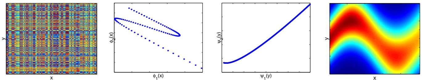
Figure 5: Reordering  $X$  and  $Y$  using SDR. From left to right: **1:** The scrambled version of  $p_2(y|x) = N(2\pi \sin x, 0.8 + 0.1x)$  **2:** Scatter plot of  $\phi_2(x)$  vs.  $\phi_1(x)$  - the  $\vec{\phi}(x)$  curved manifold. **3:** Scatter plot of  $\psi_2(y)$  vs.  $\psi_1(y)$  - the  $\vec{\psi}(y)$  manifold. **4:** Reordering of  $p_2$  according to the  $\vec{\phi}(x)$  and  $\vec{\psi}(y)$  curves.
