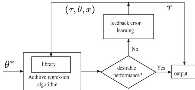
Figure 2: A schematic description of the Greedy Additive Regression (GAR) model. A desired trajectory  $\theta^*$  is given as an input to the model. An additive regression algorithm is then used to construct a torque sequence by linearly combining sequences from the library. If this algorithm fails to find a linear combination yielding good performance, the model acquires a new torque sequence by other means (e.g., via feedback error learning), and then adds this new sequence to the library.
