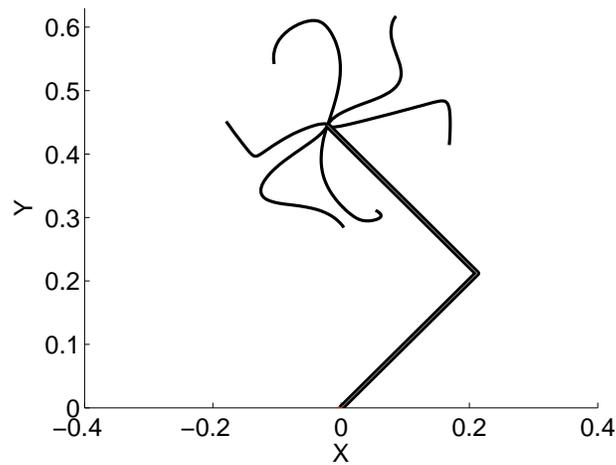
Figure 5: Cartesian-space trajectories generated by the three torque sequences that accounted for the largest percent of a GAR model’s total activation. These trajectories were generated by initializing the shoulder and elbow joint angles of the arm to  $\pi/4$  and  $\pi/2$  respectively, and then applying the sequences to the arm with coefficients of 1 and -1.
