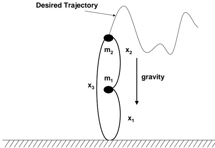
Figure 10: Schematic description of the spring-mass system used for the simulations.
