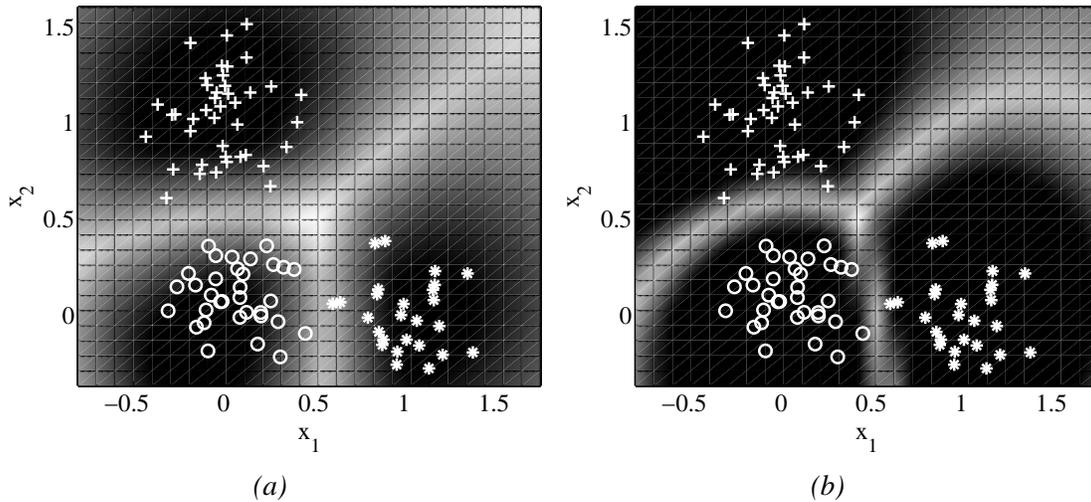
Figure 3: Equal probability contour plots for a three-class problem with the *GiniSVM* solution obtained for (a)  $\gamma = 8$  and (b)  $\gamma = 0.08$ .
