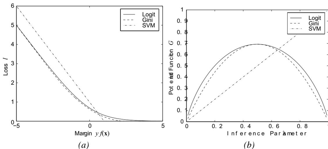
Figure 5: Primal and dual formulation of logistic regression, *GiniSVM* regression and soft-margin SVM classification. (a): Loss function in the primal formulation. (b): Potential function in the dual formulation. The *GiniSVM* loss function and potential function closely approximate those for logistic regression, while offering the sparseness of soft-margin SVM classification.  $C = 1$ , and  $\gamma = 8 \log 2$  for *GiniSVM* and  $\gamma = 1$  for logistic regression.
