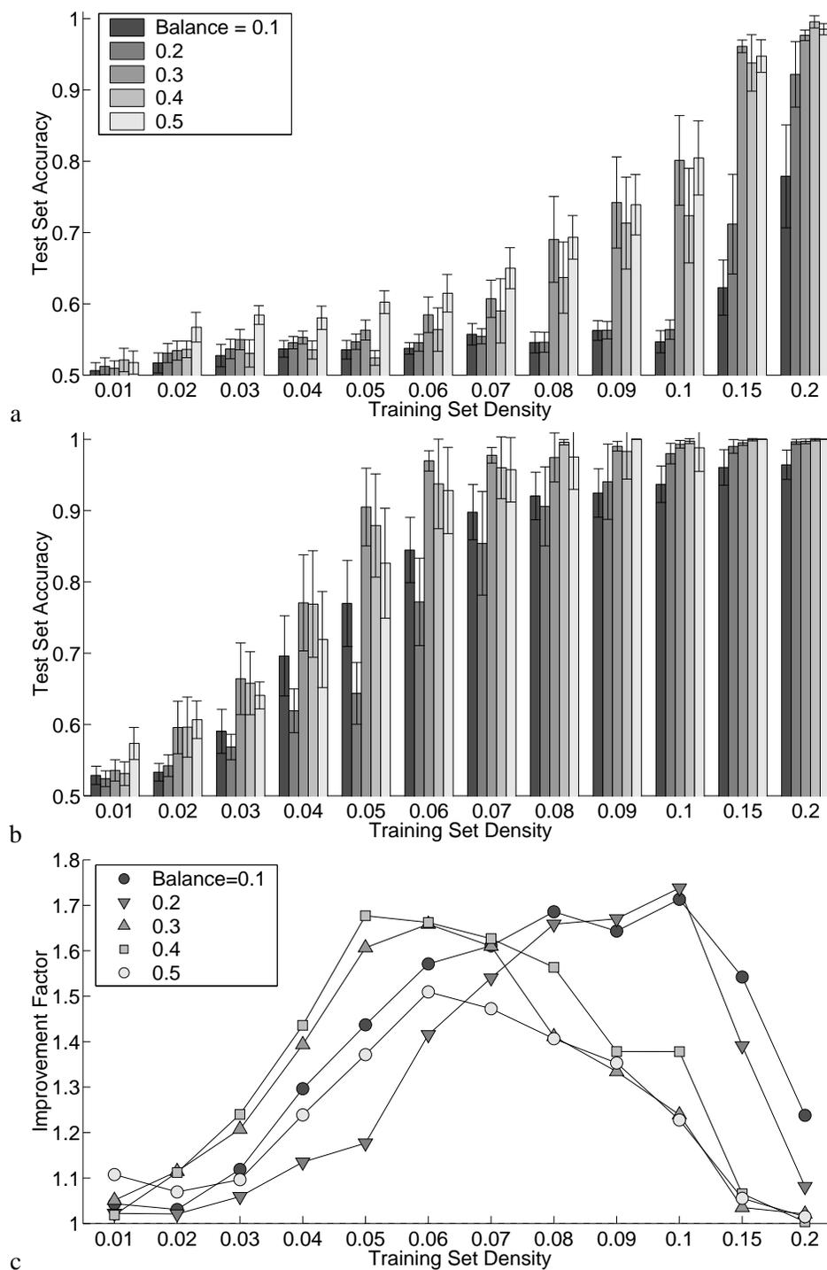
Figure 6: **Performance of the EEA against EDSM on DFAs with  $n = 16$  states and differing balances.** **a:** Mean accuracies of the EDSM for differing balances and training set densities. **b:** Mean accuracies of the EEA for differing balances and training set densities. **c:** Improvement factors of the EEA over the EDSM for differing balances and training set densities.
