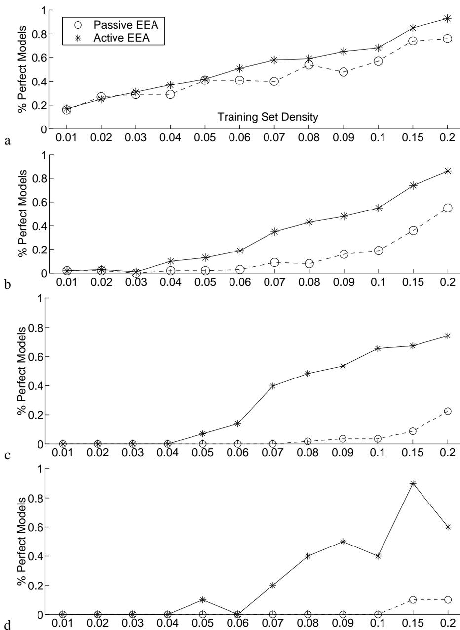
Figure 3: **Probability of Perfectly Consistent Model Discovery for the Random DFAs.** The target DFAs are grouped according to size (**a**:  $n = 4$ , **b**:  $n = 8$ , **c**:  $n = 16$ , and **d**:  $n = 32$ ) and training set density. Data points indicate the percentage of runs that produced a model that achieves 100% test set accuracy.
