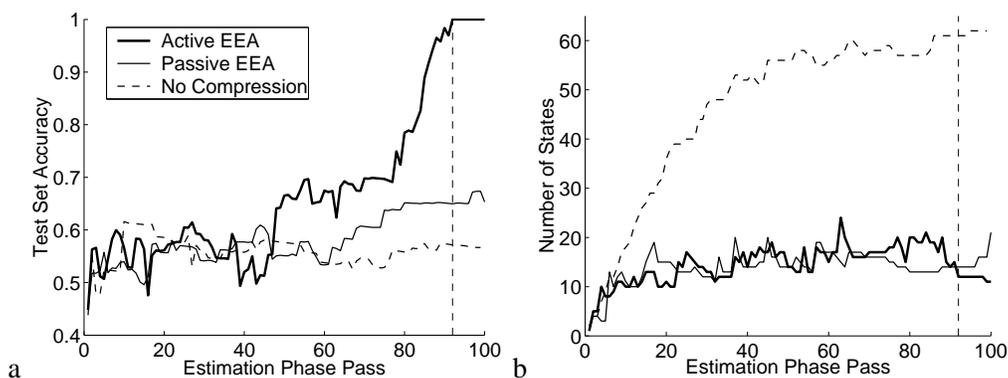
Figure 1: **Performance and Size of Candidate Models.** **a:** The test set accuracies of the best models output by each pass through the estimation phase. **b:** The total number of states used by each model when labelling the test sentences.
